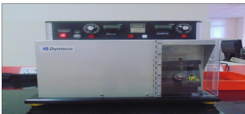
Figure 3. B.F Goodrich cutting and chipping tester
